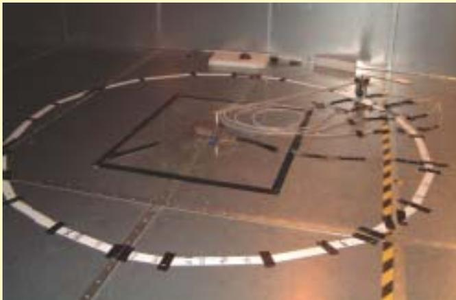
Fig 2 Vehicle simulator for Speed TLEDs with pneumatic sensors
